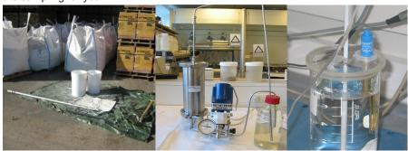
We perform accredited sampling of waste and numerous leaching tests of different materials, such as waste, residues, soil, sediments, aggregates, construction products.
