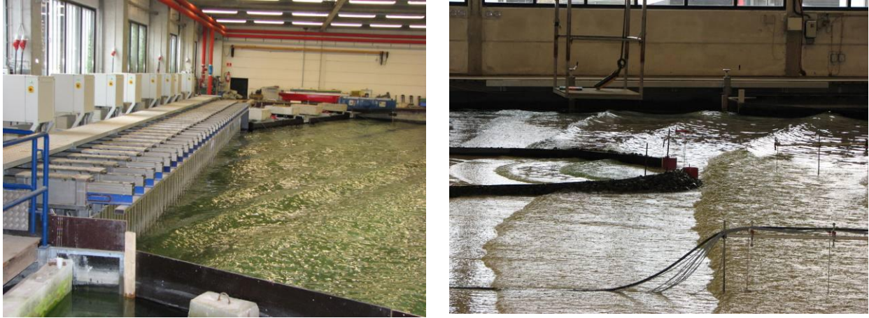
Fig. 3. DHI's shallow water basin with wavemakers (left) and harbour layout (right).
