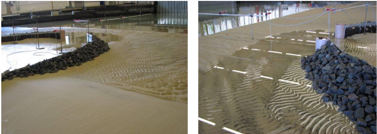
Fig. 5. Evolution of the moveable bed experiment: upstream sedimentation (left) and bypass bar with down-drift erosion (right).
