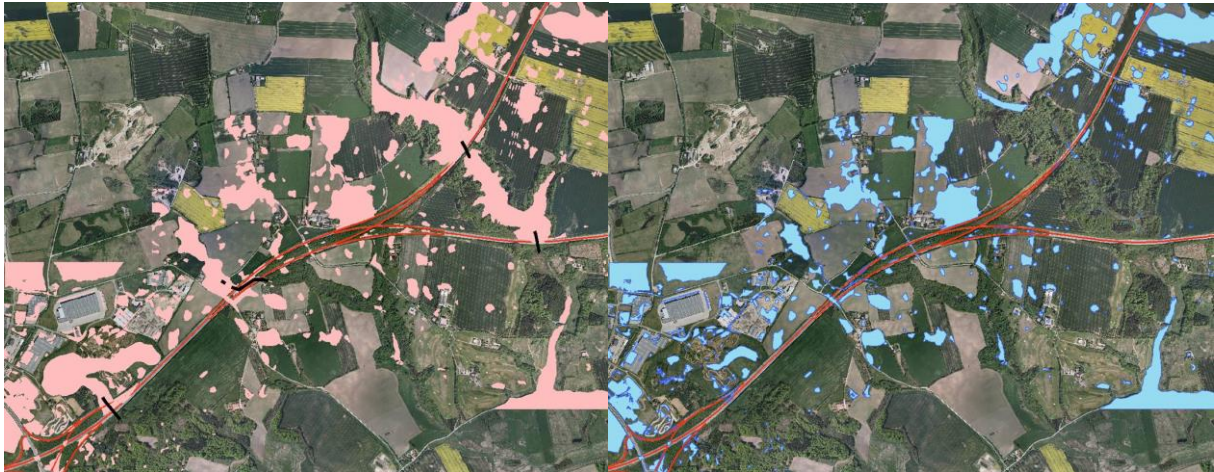
Figure 3.2 Calculated depressions before culverts are opened (left) and after having been opened up (right). (Vejdirektoratet, 2009)
