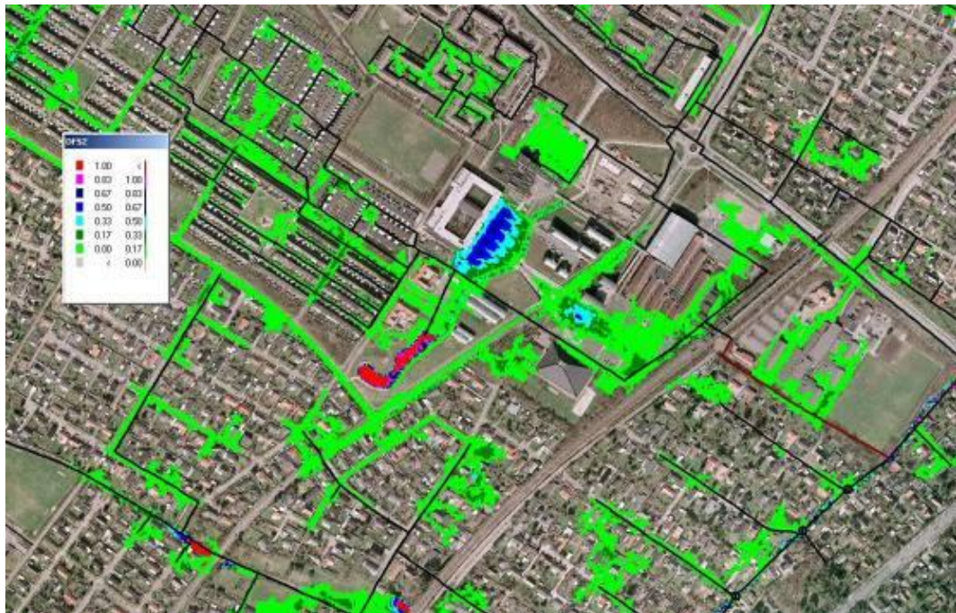
Figure B. 7 Max. Flooding depths calculated for a 10-year CDS rainfall, extrapolated by 100 years. Input: 10-year CDS rainfall and water level in Køge Bay extrapolated for climate scenario A2
