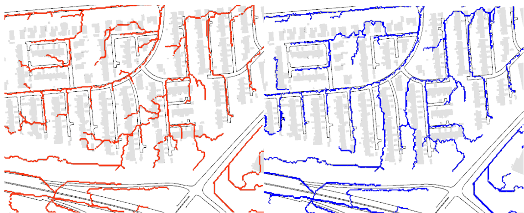
Figure 3.5 Waterways on the surface calculated without houses (left) and including houses (right)
