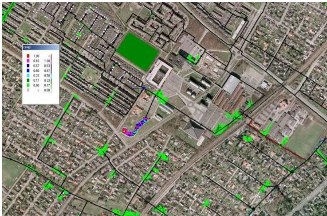
Figure B. 11 Max. water levels after installation of two 0.5 m 3 /s pumps and utilisation of the football field as rain water basin. Reference calculation is shown in Figure B. 6. Input: 10-year CDS rainfall and water level in Køge Bay extrapolated for climate scenario A2
