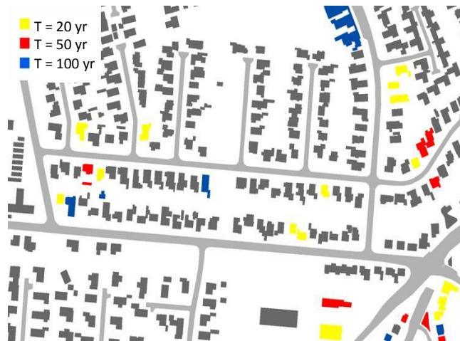
Figure 5.4 Example of GIS theme of the houses flooded at different return periods
