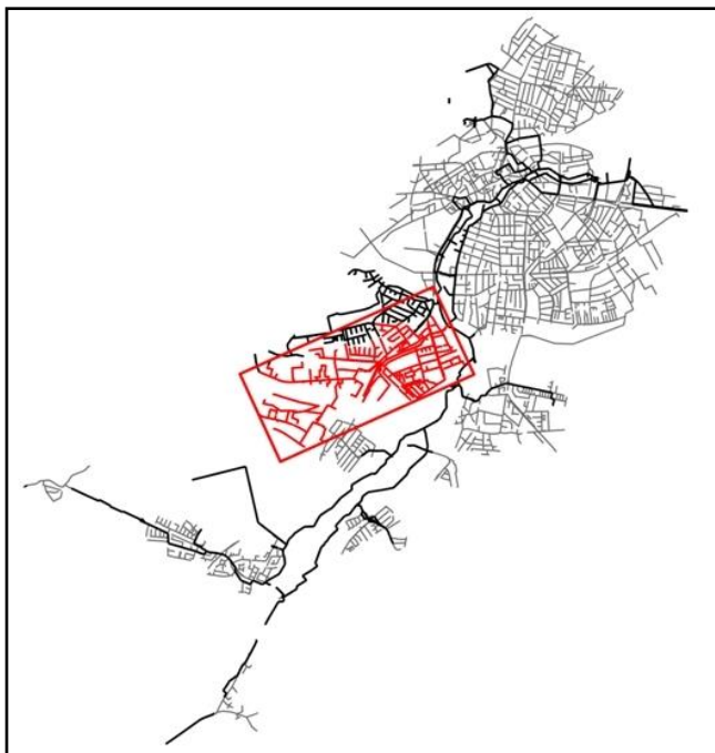
Figure 3.20 Collection system model coupled to 2D terrain model
