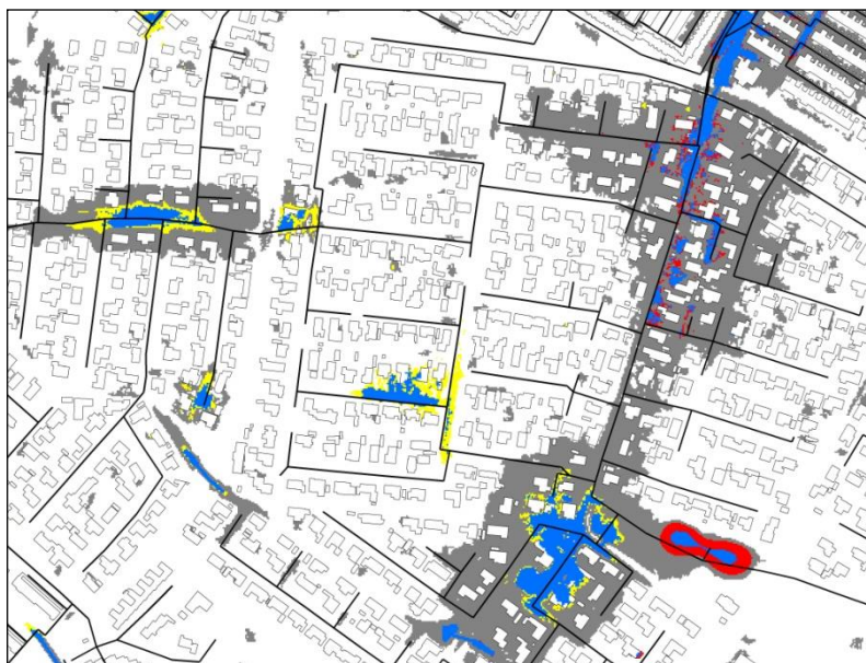
Figure 3.24 Correlation between results of Depression Method (grey), hydraulic surface calculation (red) and combined hydrodynamic drainage model and surface model 1D-1D (yellow) - Blue coincide hydraulic surface calculation and combined hydrodynamic drainage model
