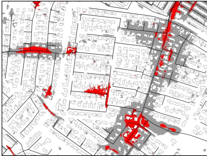
Figure 3.12 Example of flood results when hydraulic surface charge of 100 years of rain (red) compared with Depression Method (grey)
