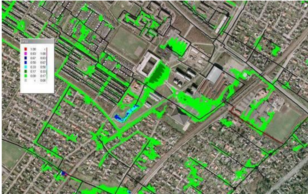
Figure B. 6 Max. flooding depths calculated for a 10-year CDS rainfall extrapolated by 10 years. Input: 10-year CDS rainfall and water level in Køge Bay extrapolated for climate scenario A2
