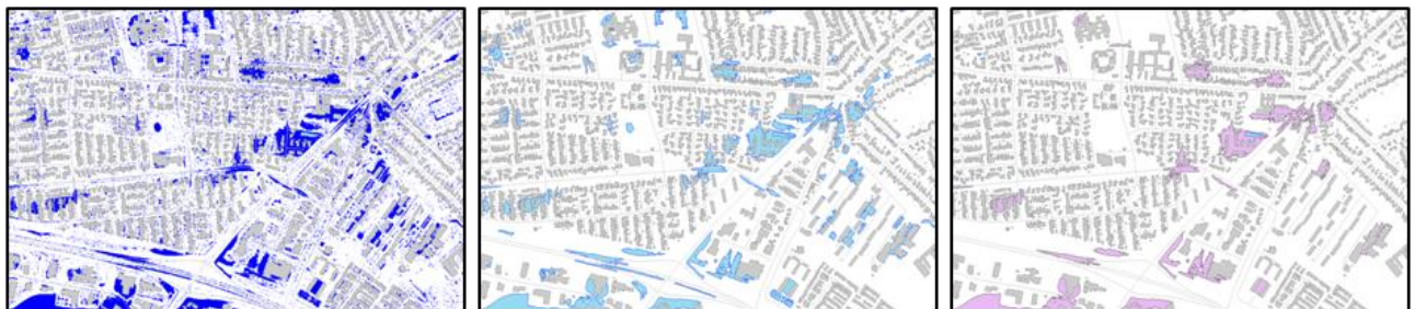
Figure 3.3 Reduction in the number of depressions based on volume. The first part shows all depressions, the second part shows depressions of 100 m 3 and the third part shows depressions over 500 m 3
