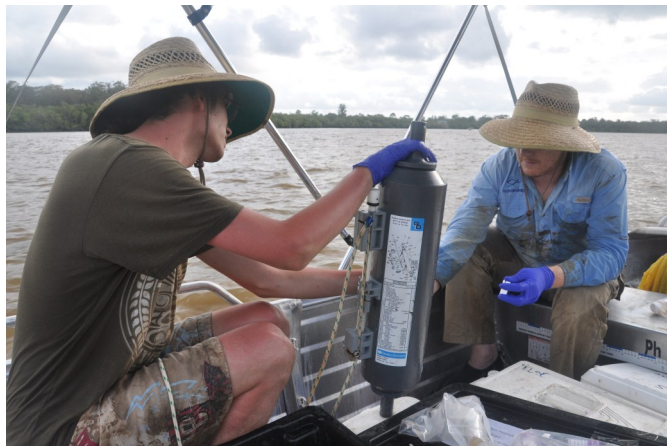
Installation of a water sampler in the Mary River during a field trip.
