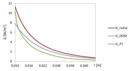
Different models for UV intensities produce significant variations in radial UV distribution
