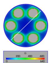
UV intensity in six-lamp reactor (cross-section)
