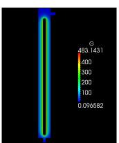
Contours of UV field intensity in a BW reactor with one UV lamp
