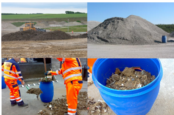
Sampling of shredder waste to determine the recovery potential
